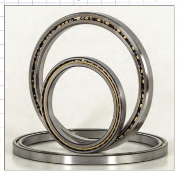
Most radial ball bearings are designed so that as the bore size increases, the width and the thickness of the bearing changes proportionately. Thin section bearings reduce total cost in a system because the cross section remains the same as the bore diameter increases, thereby improving design efficiency over standard bearing geometries.
